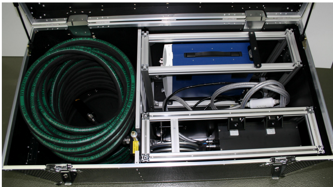
Image showing location of laser module, ICE 450 module and fibre-optic umbilical inside transit case
