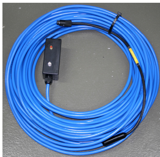
CAD image of submersible remote monitor housing (left) and image of underwater connecting cable / umbilical (right)
