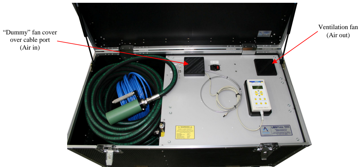
Image showing LIBSProbe components installed inside transit case
