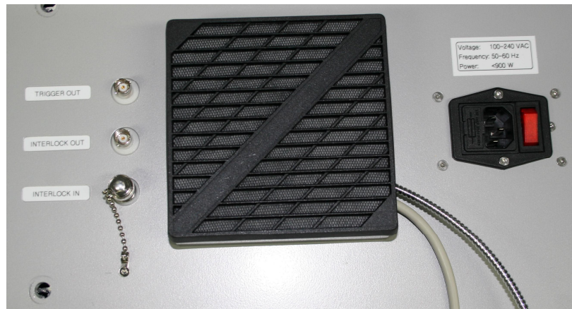
Image showing “snap fit” fan cover fitted to cable port in top cover
